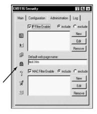
The *Default web page name* lets the Administrator specify an addition to the IP address that the user must include when he accesses the KN2108 / KN2116 with a browser. For example:
